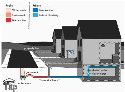
water pipe material entering home. This determination should be made where the service line enters the house, most likely through a basement wall and before the water meter. Not sure on pipe material type? Use the chart below to assist in determining. Still need help? Contact the Borough Office to schedule an appointment with the Water Department.
