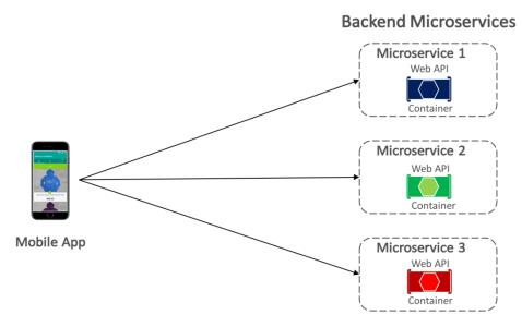
With direct client-to-microservice communication, the multi-platform app makes requests to each microservice directly through its public endpoint, with a different TCP port per microservice. In production, the endpoint would typically map to the microservice's load balancer, which distributes requests across the available instances.
