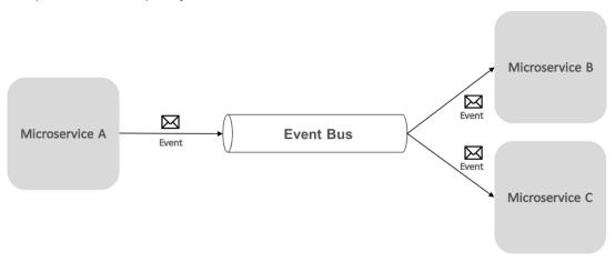
From an application perspective, the event bus is simply a publish-subscribe channel exposed via an interface. However, the way the event bus is implemented can vary. For example, an event bus implementation could use RabbitMQ, Azure Service Bus, or other service buses such as NServiceBus and MassTransit. The diagram below shows how an event bus is used in the eShopOnContainers reference application.
