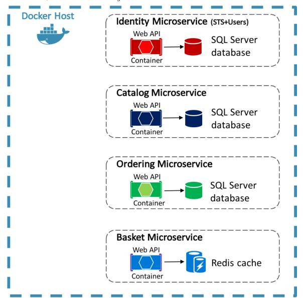
The architecture of the back-end services in the reference application is decomposed into multiple autonomous sub-systems in the form of collaborating microservices and containers. Each microservice
